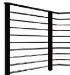
4 custom railing: dark grey 2"x3" tube steel frame with 5/8" metal rod infill height 36" posts: 3"x2" dark grey tube steel height 8'-0"
